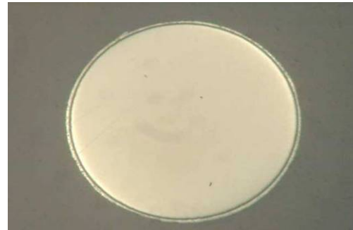
EMW controlled zinc application
