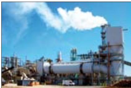
The new woodchip drier at the Laminex site in Dardanup, Australia, commissioned in December 2006.
