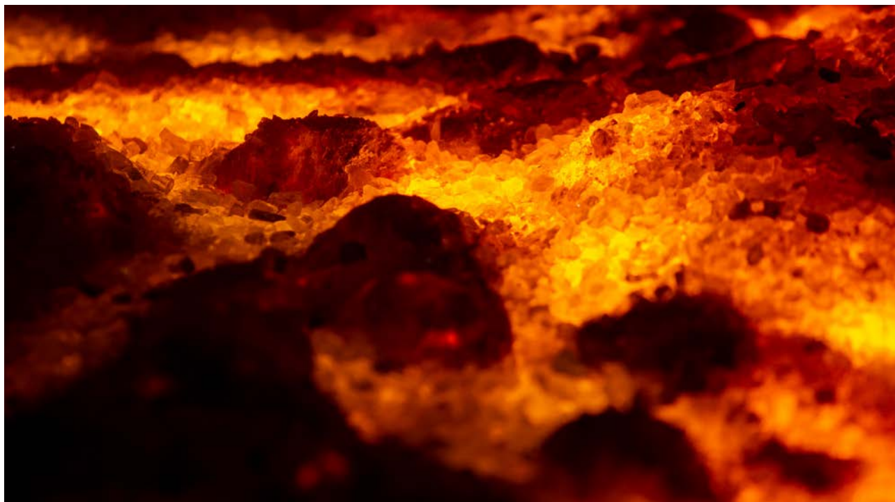
Recycled glass is melted down at Tasman Insulation to make Pink® Batts®
